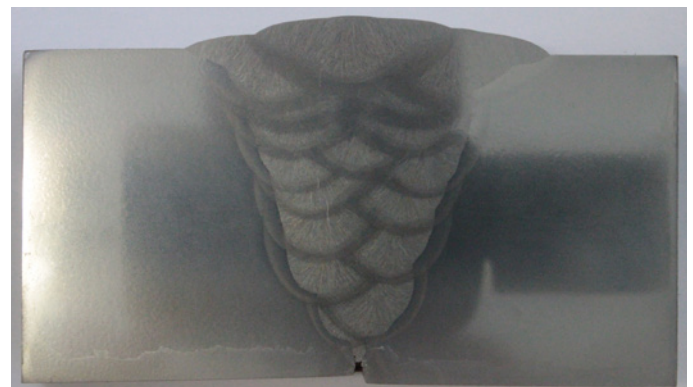
3-Wire Spitfire Welding Process
