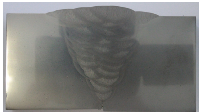
3-Wire Reference Welding
